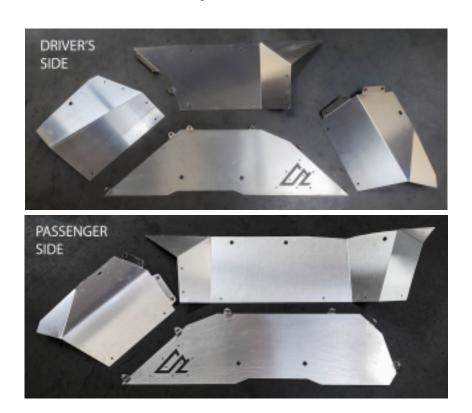
2.) Using (13Driver, 10Pass) M6 x 14mm Button Head bolts and a 4mm allen socket, assemble the panels into a unit. Leave these bolts loose until final assembly. The assemblies should look like the images below.
